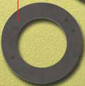
Radial cut front ring allows air into the seal chamber via the gaps thus pressure actuating the tangent cut seal ring onto the piston rod
