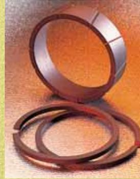
The larger 1st and 2nd stages should normally use CPI piston ring styles A00 or A01, which are both single piece designs. The A00 type is straight cut and is specified for aluminium pistons where spinning rings are known to cause piston groove wear. CPI also recommends that the piston groove flanks are hard anodised as standard to
